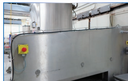
HYGIENICALLY DESIGNED SLOPED SURFACES FOR WATER RUNOFF
