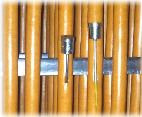
Figure 3 – Comparison of internal measurement and surface measurement in snack sticks
